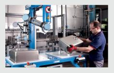
**Result:** Swiss kitchen manufacturer Franke uses a UR5 cobot to streamline its production of kitchen sinks, precision-gluing mounting blocks on each side. The UR5-based setup has been in non-stop operation since November 2011, producing more than 10,000 sinks a year. The cobot ensures that the pressure applied, the amount of glue used and the overall quality of the gluing process are all consistent.
